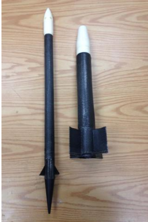
Figure 2. Dart and Booster . These are the first version of the dart and booster with the ABS transition and nose cone pieces.
