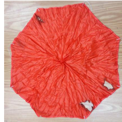
Figure 4. Post-Testing Parachute . Ground testing of descent control ejection taught us that the parachute needs Nomex protection from the ejection charges
