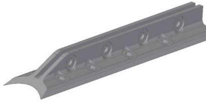
**Figure 4<sup>1</sup>. Sustainer fin bracket** *The booster and sustainer fin brackets are very similar and will both be 3D printed from ABS.*
