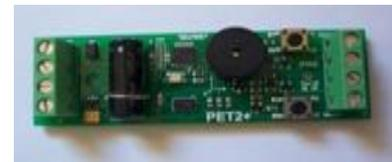
**Figure 10. PET2+ Timer** The Pet2+ Timer made by Missile Works will control second stage ignition.
