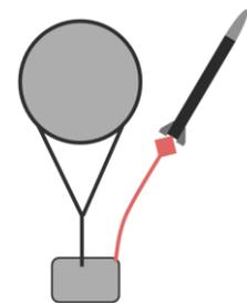
**Figure 9. Rockoon diagram** *Basic concept of operations for a rocket launching from a high-altitude balloon.*
