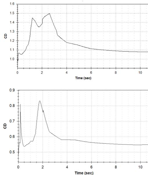
**Figure 7. CD vs Time Data for Mach 6 (top) and Gold Team (bottom) during flight from RAS Aero II**
