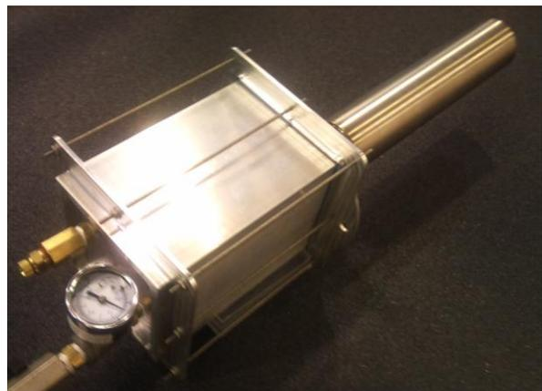
Figure III: Neutron Counter Payload during pressure test.
