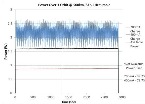
Fig. 2: (Blue) Solar power available at beginning of life (BoL) to ChargerSat-1, a 1U CubeSat, over one orbit. Model developed using data generated in STK. This chart does not show eclipse operations. The red and black curves represent the power required to charge a Li-Po battery, starting at 40% state of charge (SoC), at 200mA and 400mA CC respectively. Charging power data collected experimentally.
