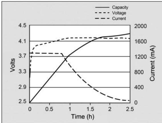
Fig. 1: Capacity as a function of charge voltage on a lithium-ion battery<sup>1</sup>.
