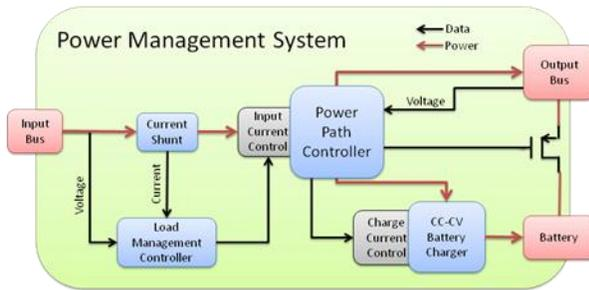
Fig. 3: Block diagram of the power management system in its simplest form. Power is sourced from the input bus at 4.5-5.5V. Black arrows represent data and red arrows represent power flow.
