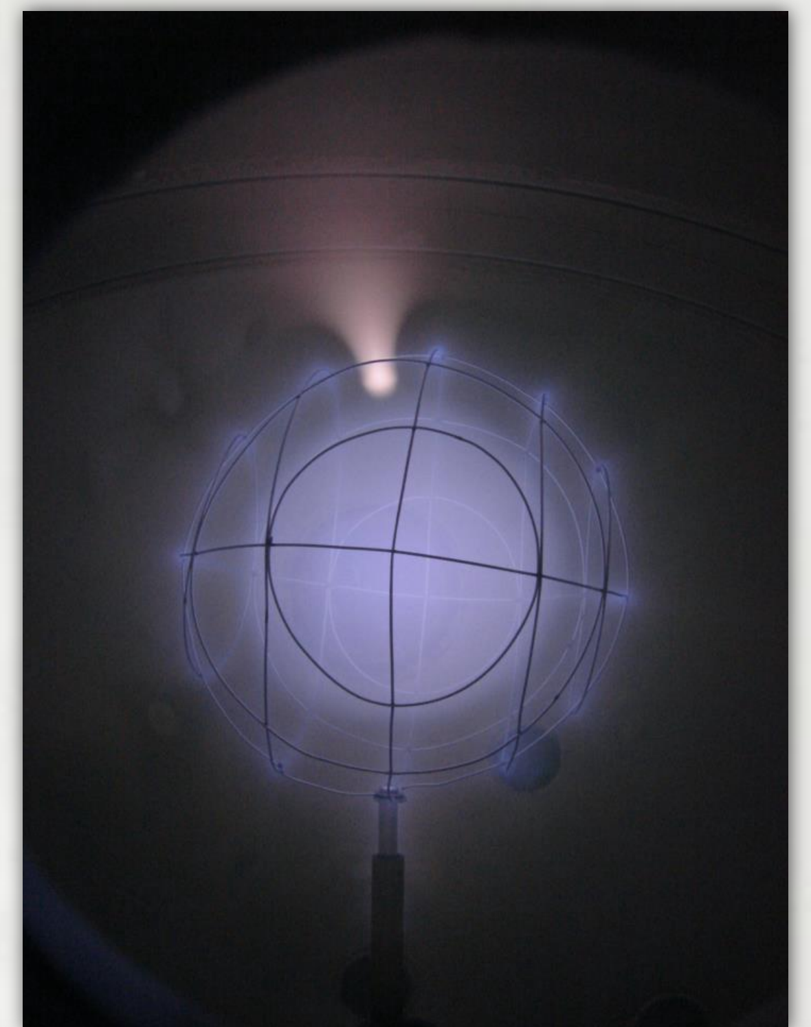
IEC Reactor, Argon, 2kV and 50mA Inner electrode through viewport MSFC ER-24
