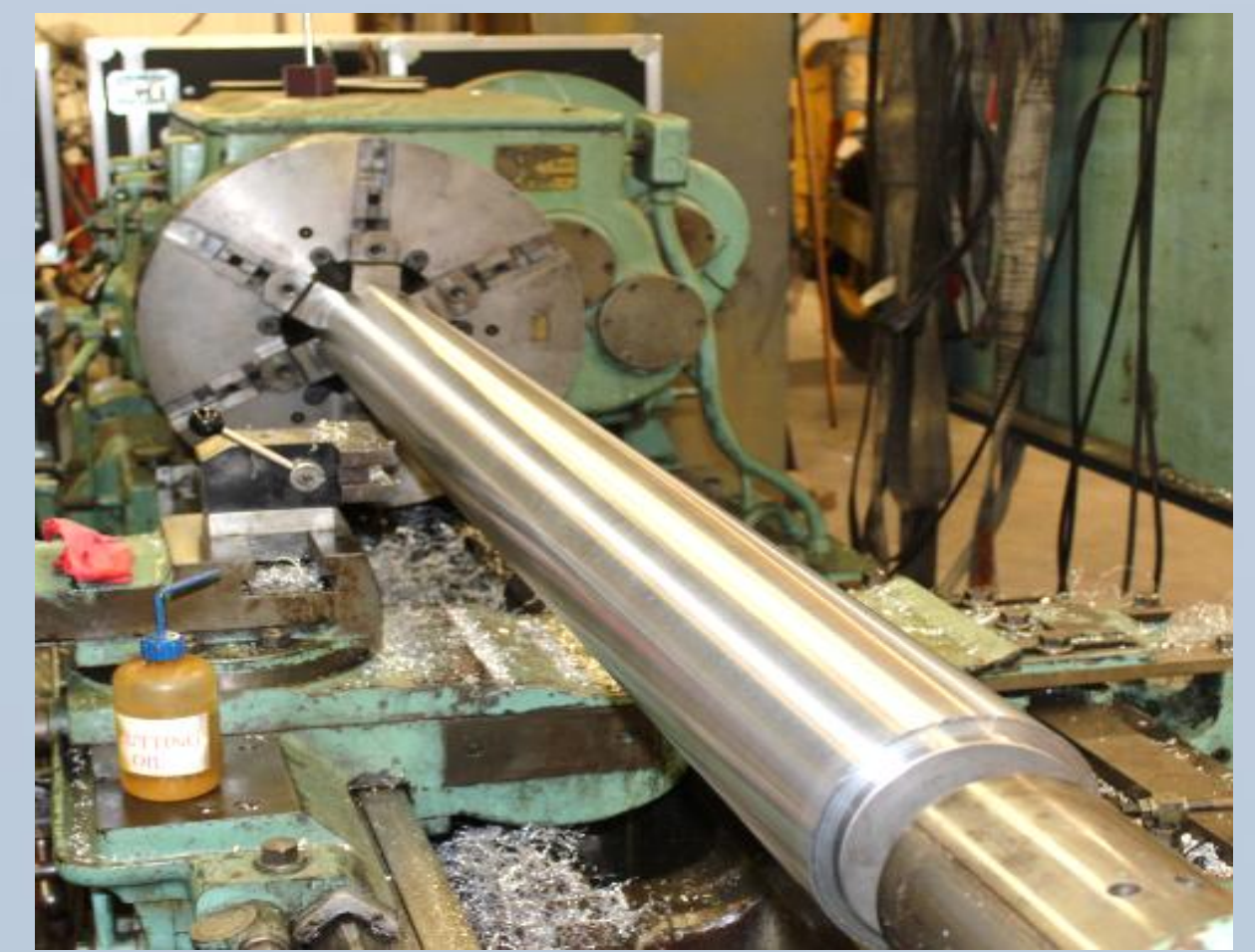
6" x 6' mandrel for composite rocket body layups
