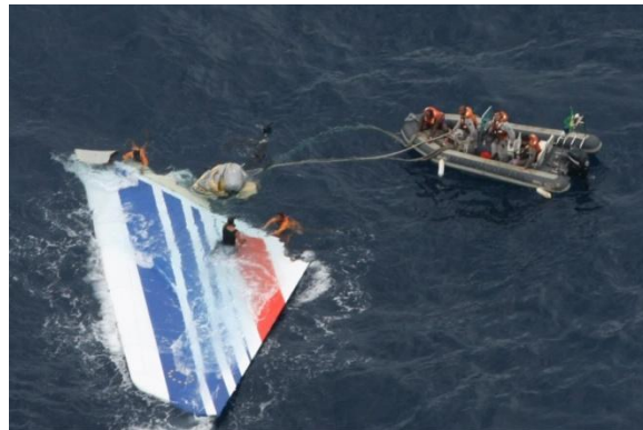
Figure 8: The vertical stabilizer of Air France flight 447 being recovered from the Atlantic within a few days of the crash.
