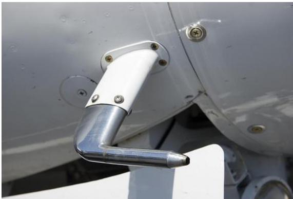
Figure 7: A pitot tube on a small aircraft. Although most pitot tubes are heated, there have been instances when they have iced over.
