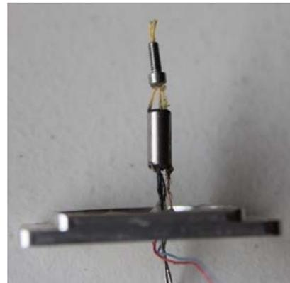
Fig. 1: The test sample mounted to the base of the chamber with the upper suspending cords attached. Electrical leads for current and temperature are seen passing through the base.
