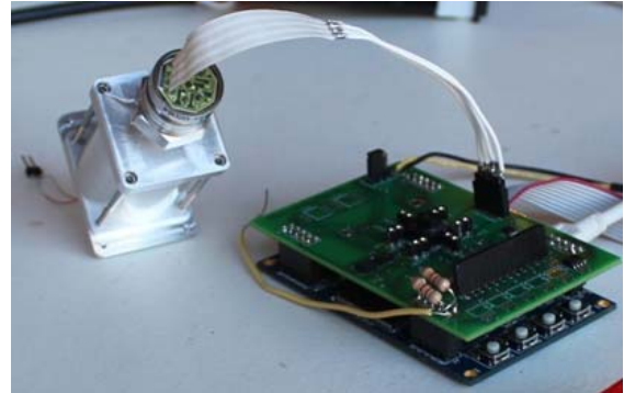
Fig. 3: The experimental chamber set up with the pressure sensor attached to the PCB with its needed ADC.
