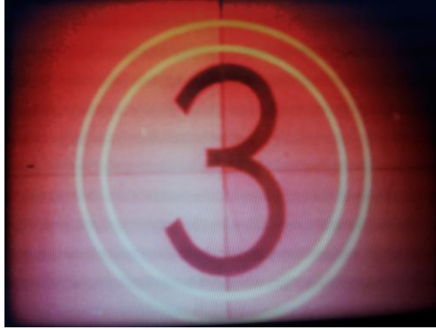
Fig. III: Horizontal lines are visible when the refresh rate of the projector and receiver are not fully in phase. These lines appear to move slowly down the screen.
