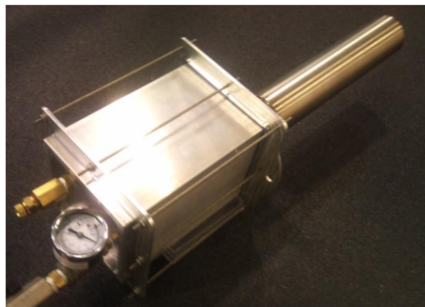
Figure III: Neutron Counter Payload during pressure test.
