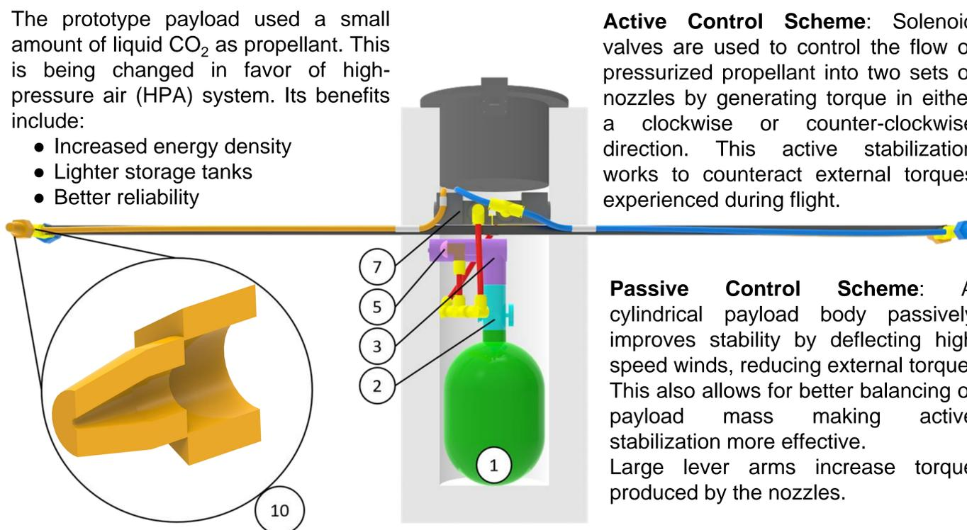
**Active Control Scheme:** Solenoid valves are used to control the flow of pressurized propellant into two sets of nozzles by generating torque in either a clockwise or counter-clockwise direction. This active stabilization works to counteract external torques experienced during flight.
