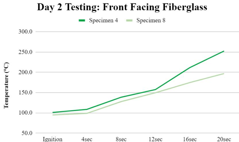
**Figure 8: Comparison of 3 and 4 layer Front Facing Fiberglass Specimens.**
