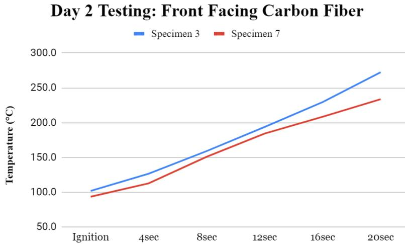
**Figure 9. Comparison of 3 and 4 layer Front Facing Carbon Fiber Specimens**
