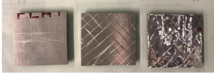
**Figure 4. Unfinished, Diamond, and Rough Surface Finishes**
