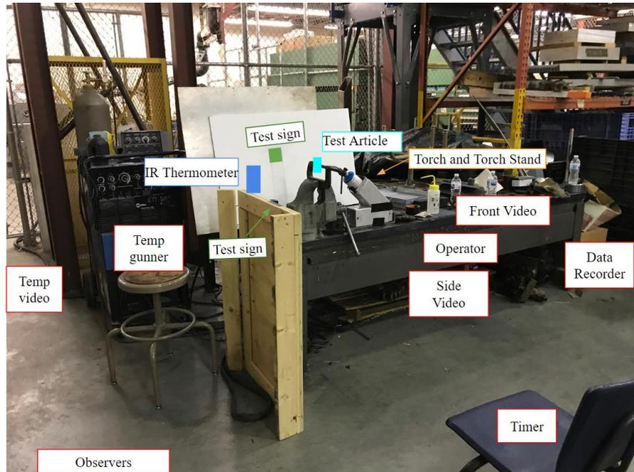
Figure 3. Labeled Image of Testing Setup
