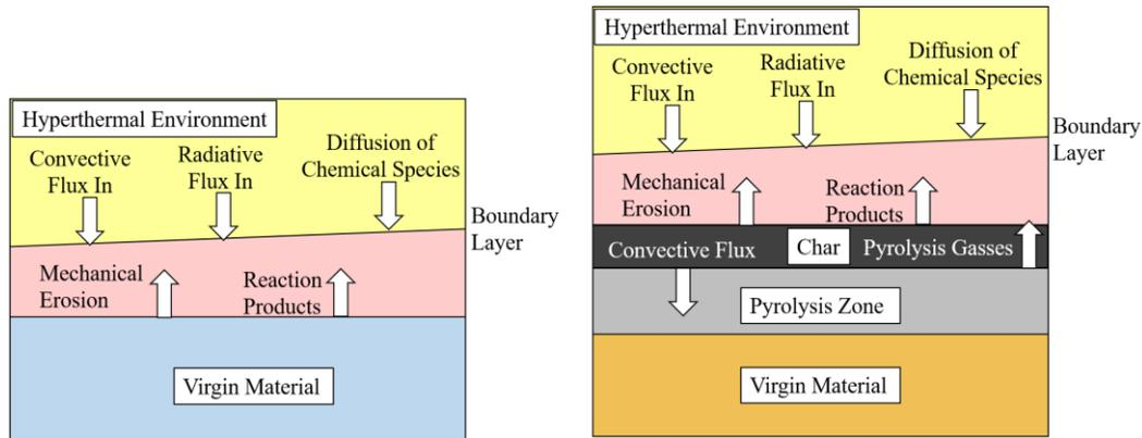
**Figure 1. Diagram of Polymeric Ablative Process<sup>1</sup>**
