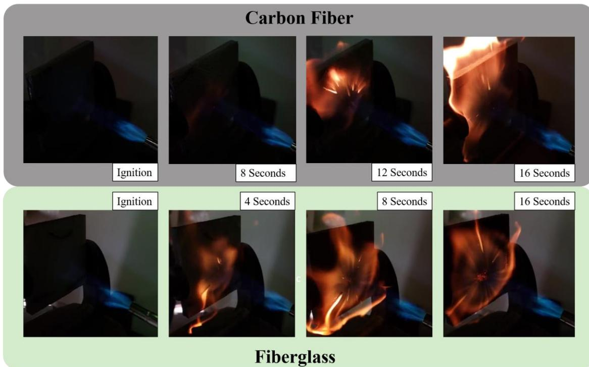
**Figure 10. Comparison of Images During Carbon Fiber or Fiberglass Trials**
