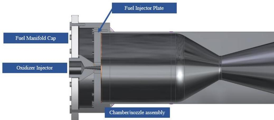
**Fig. 4 Preliminary Engine Render with Labels**
