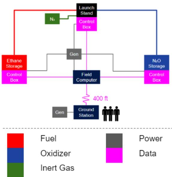
**Fig. 2 Block Diagram of Preliminary Ground System**
