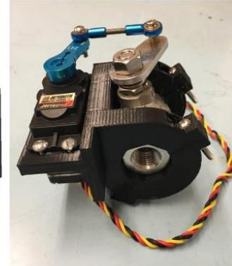
**Fig. 7 Render and Development Hardware of Servo-Driven Ball Valve**
