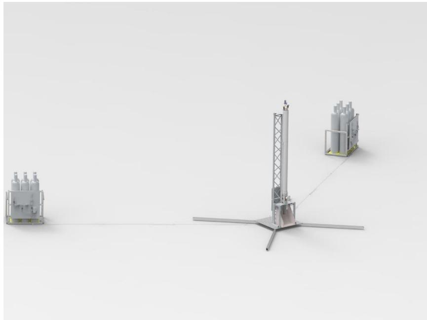
**Fig. 1 Render of Field Layout with Test Structures**
