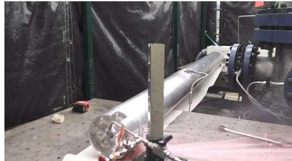
**Fig. 15 Rupture During Hydrostatic Testing**
