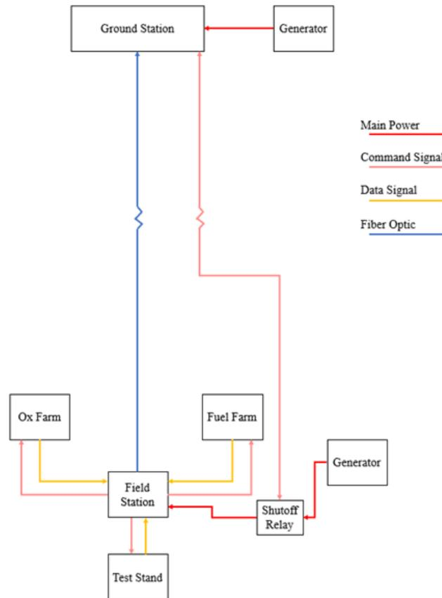
**Fig. 12 Updated Ground System Power and Data Block Diagram**
