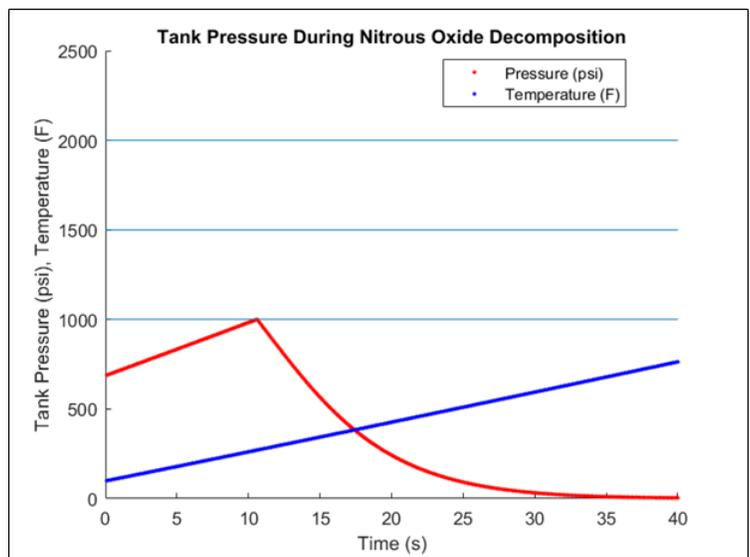
**Fig. 14 Results of Nitrous Oxide Decomposition Model**
