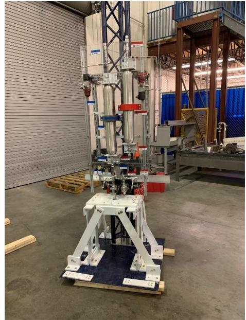
**Figure 1. Tartarus' main fluid panel and hold down**
