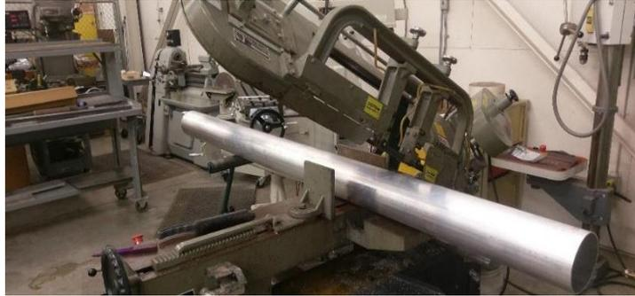
**Fig. 6 Pressure Vessel Cylinder on Horizontal Band Saw**
