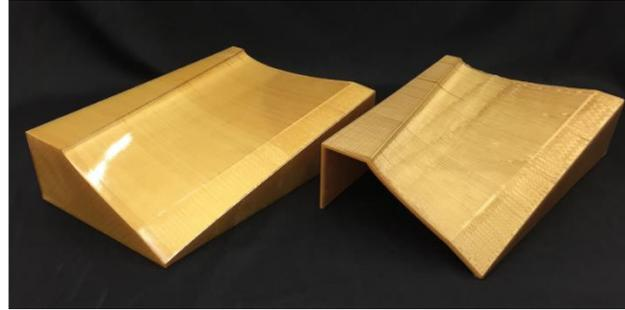
**Fig. 3 3D Printed Molds from Stratasys Tooling Design Guide [3]**
