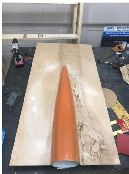
**Fig. 6 Plug Placed in Parting Board**
