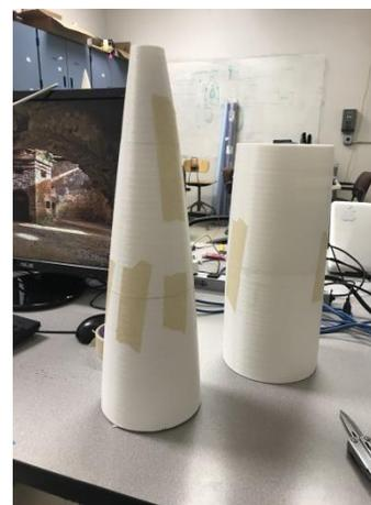
**Fig. 5 Printed Plug During Assembly Process**
