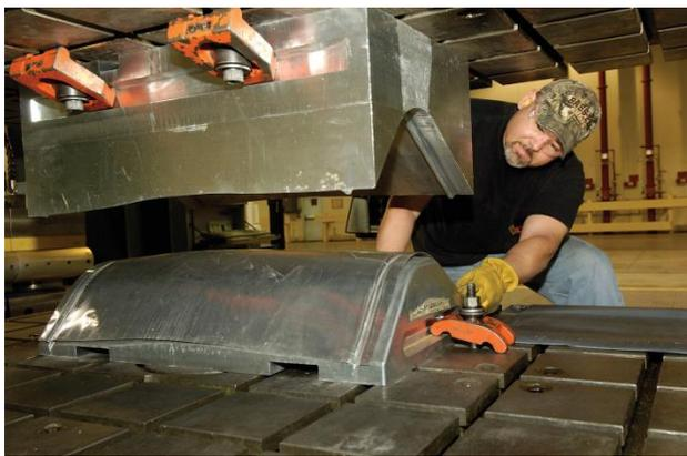
**Fig. 2 Industrial Male- Female Mold <sup>[2]</sup>**
