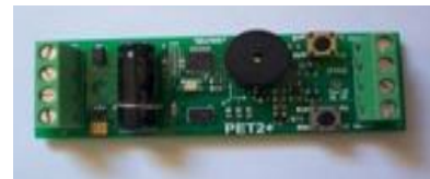
Figure 10. PET2+ Timer The Pet2+ Timer made by Missile Works will control second stage ignition.
