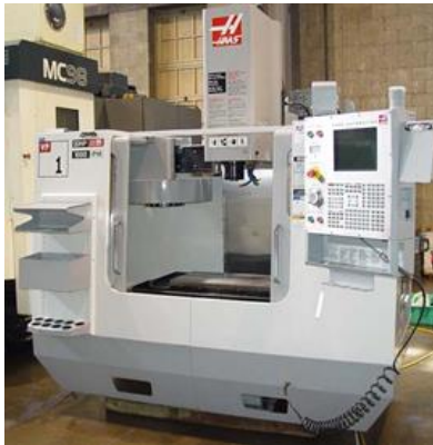
Figure 15. Haas VF-1 The Haas VF-1 in the UAH MAE EDPF is used to manufacture all CNC milled parts for Project URSA.
