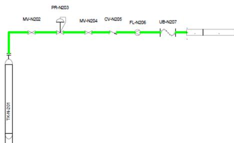
**Fig. 14 GSE Pressurant System**
