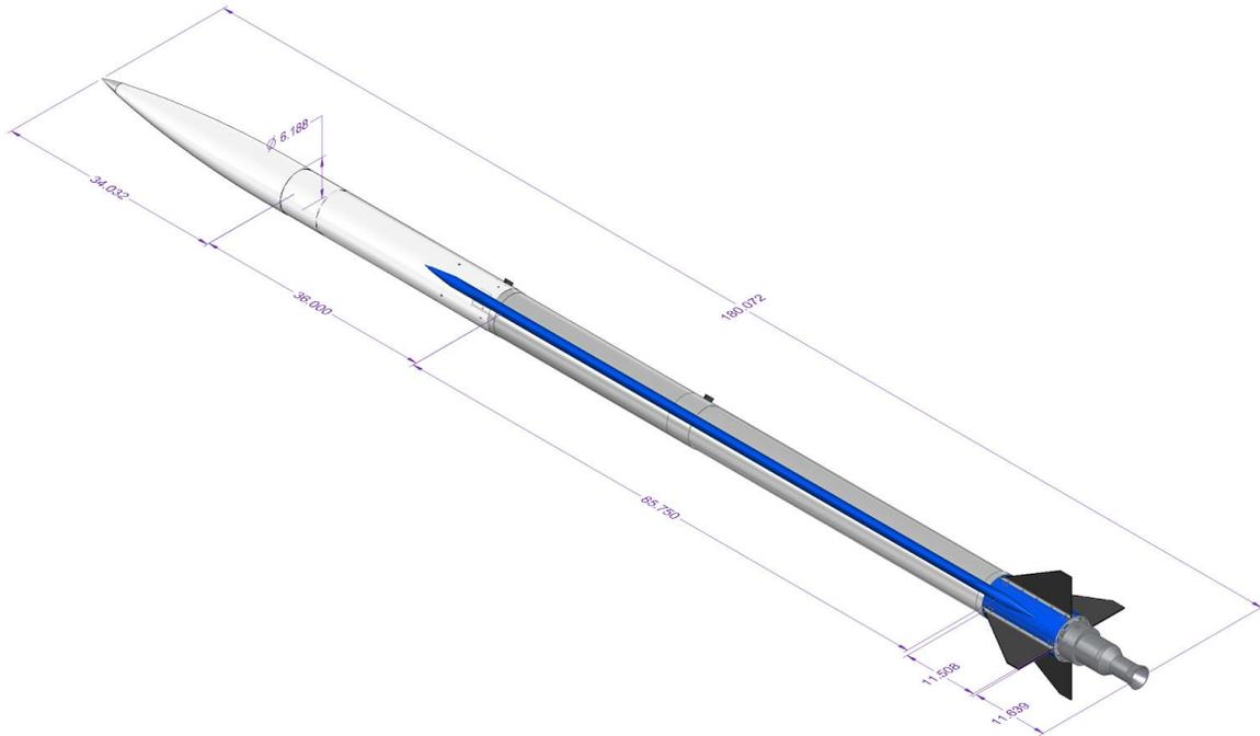
**Fig. 1 Dimensioned CAD of overall rocket (inches)**
