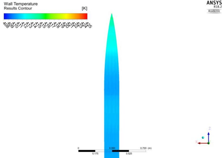
**Fig. 7 Nose Cone Adiabatic Temp. Dist. at M1.44**
