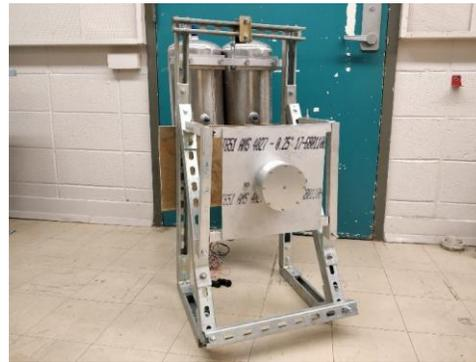
**Fig. 15 Cold Flow Stand w/ Workhorse Cold Flow Test Article**
