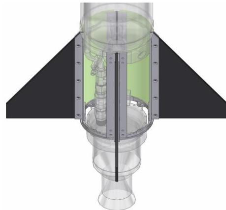
**Fig. 5 Thrust Assembly and fin attachment**
