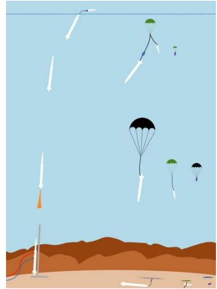
Fig. 6 Launch and Recovery Concept of operations
