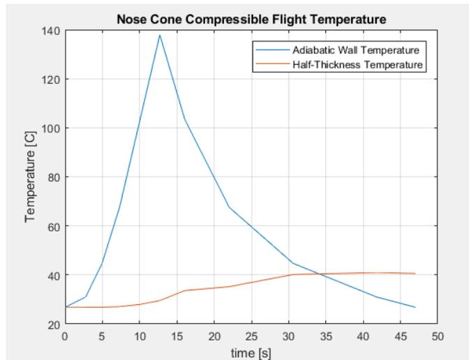
**Fig. 8 Nose Cone temperature distribution vs time**
