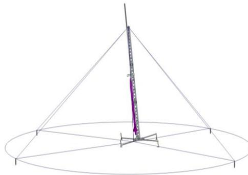
**Fig. 10 GSE test stand with integrated rocket**
