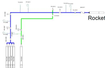
**Fig. 13 GSE Nitrous Oxide System Schematic**
