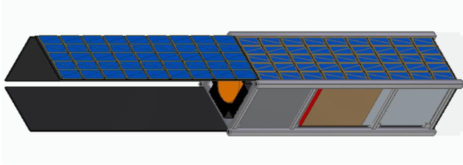
**Fig. 2 Overview of the spacecraft (external view, one side of baffle is removed for clarity).**
