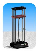
In course work, my senior design project was to design a piece of lab equipment the department uses to this day. The equipment is a column buckling apparatus that compresses structural elements though their peak load to demonstrate the engineering calculation accuracy. The equipment improved the testing setup and provided experimental results greater than 80% of theoretical. Previous off-the-shelf systems provided less than 40% of anticipated results.
