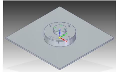
**Figure 2:** Third design of the Particle Deflector showing the change in center section and hub as well as the change in outer dimensions
