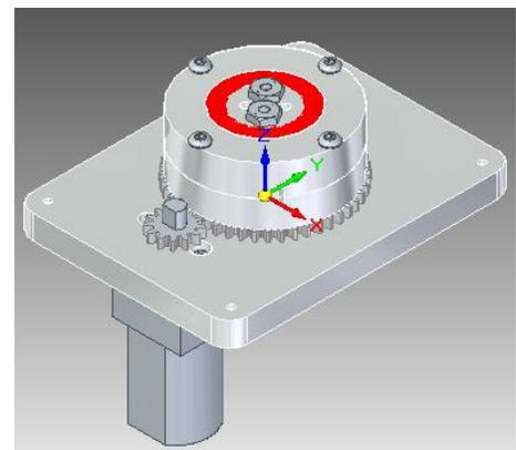
**Figure 3:** Current design of the particle deflector with a smaller plate and added motor and gear system.
