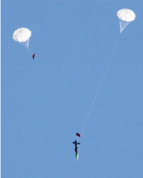
**Figure 9. Descent under both parachutes during January test flight**
