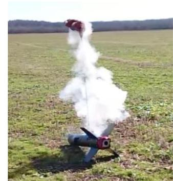
**Figure 11. Parachute deployment testing**
