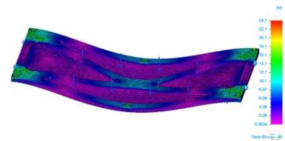
Figure 3. FEA of Rover Chassis
