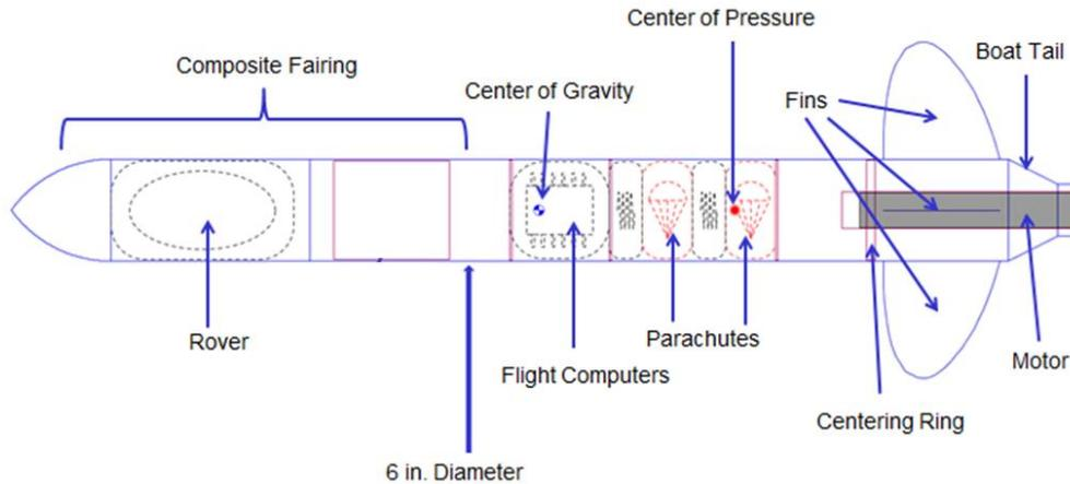
Figure 5. The layout of major rocket components
