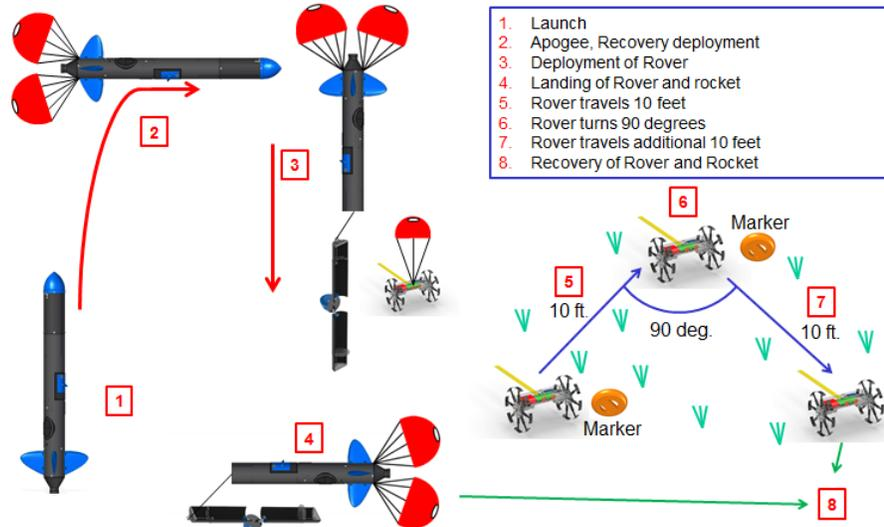
Figure 2. System Concept of Operations
