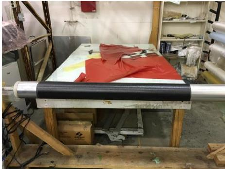
**Figure 10. Body tube preparing for cure on the mandrel**
